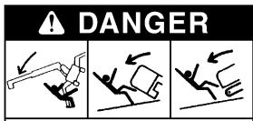
When the machine inclines in excess of 3 degrees during crane work, or in excess of 15 degrees during travel, the tipping alarm buzzer will sound. For preventing it from tipping over, return it to the state for the buzzer not to sound at once, and start the work or traveling.
