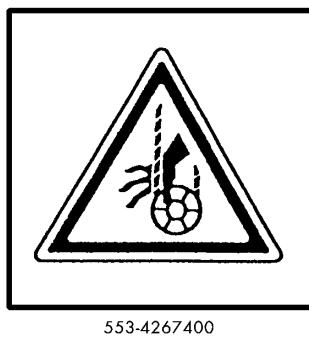
(25) Caution against being entangled by the hook block (553-4267400)
