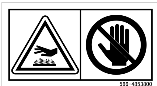
(40) Cautions against the risk of burns in the engine room (586-4853800)
