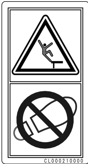
(18) Cautions on the fenders (CL000210000)
