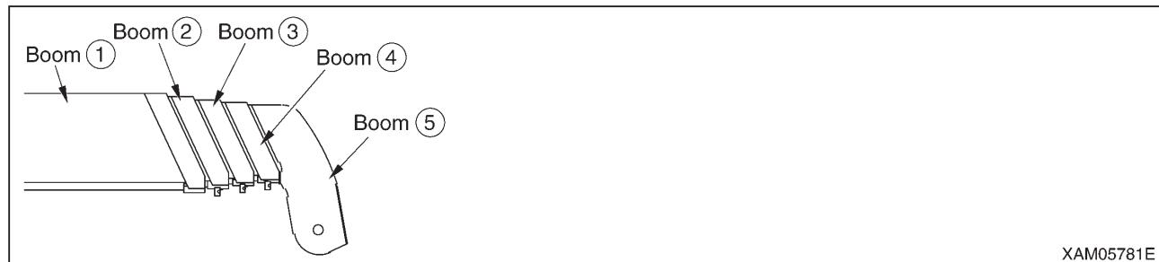
2. "Boom (1) + (2)": With booms (3), (4), and (5) retracted, boom (2) is fully extended.
